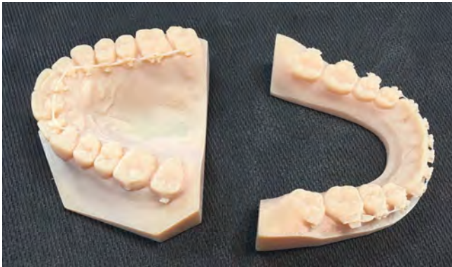
Figure 2 These dental models were fabricated through intraoral scanning and 3D printing.
